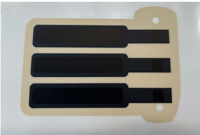
Figure 2: EMG electrodes screen printed with the conductive ink on a PU substrate with a screen printed cover of the barrier ink.
